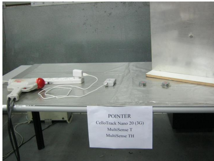
Figure 15. Immunity to Electrostatic Discharge Test
